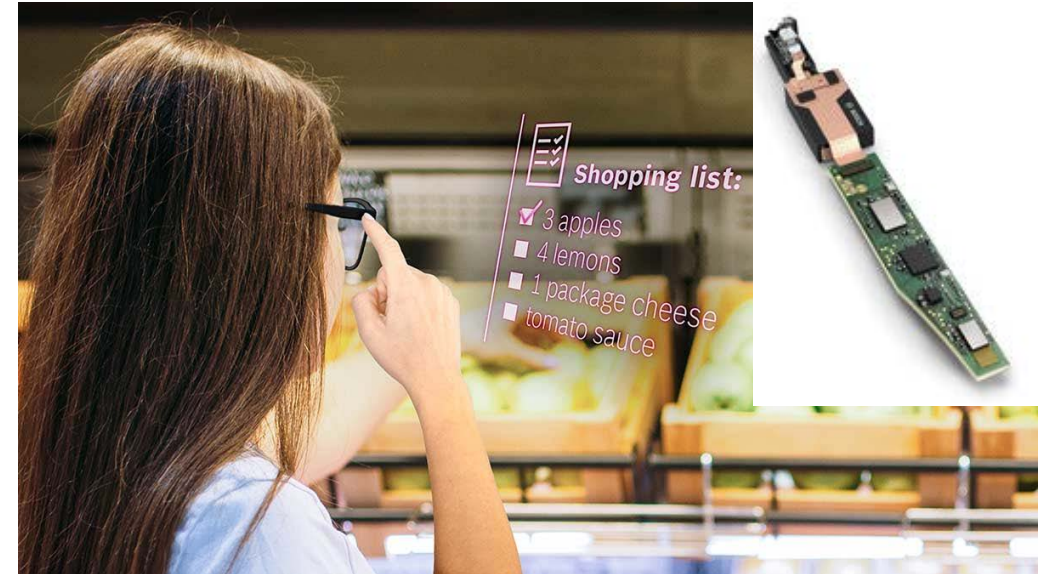
Smart glasses with \mu -mirror based projection
