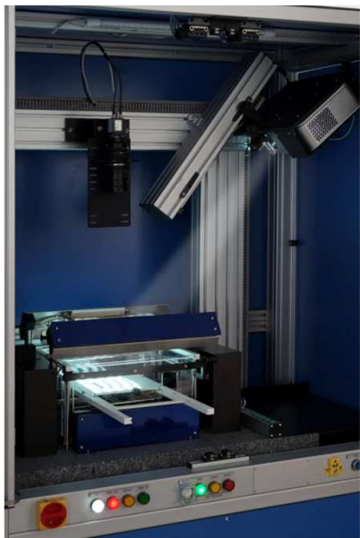
Equipment ("TDM Compact") used for warpage measurements
