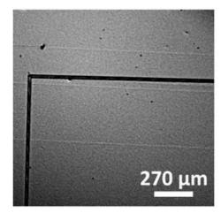
Bowing or cracking of GaAs films on Si
